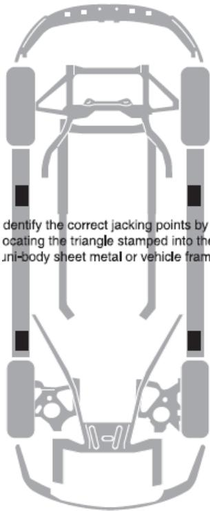
Identify the correct jacking points by locating the triangle stamped into the unibody sheet metal or vehicle frame.
