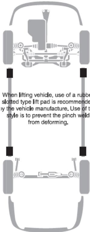
When lifting vehicle, use of a rubber slotted type lift pad is recommended by the vehicle manufacture. Use of this style is to prevent the pinch weld from deforming.
