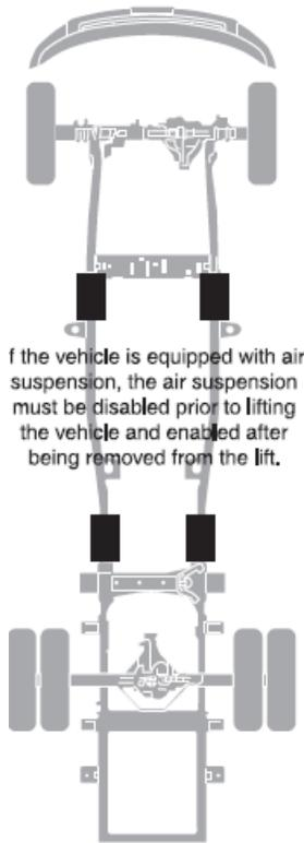
If the vehicle is equipped with air suspension, the air suspension must be disabled prior to lifting the vehicle and enabled after being removed from the lift.
