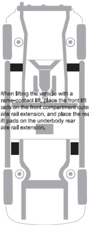
When lifting the vehicle with a frame-contact lift, place the front lift pads on the front compartment outer side rail extension, and place the rear lift pads on the underbody rear side rail extension.
