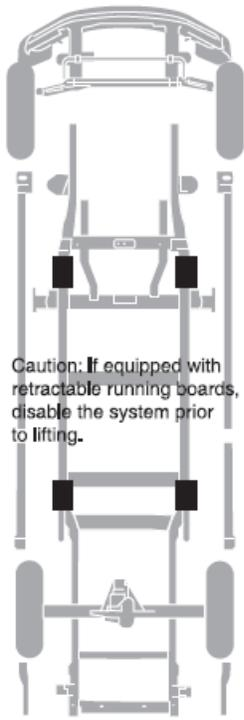
Caution: If equipped with retractable running boards, disable the system prior to lifting.
